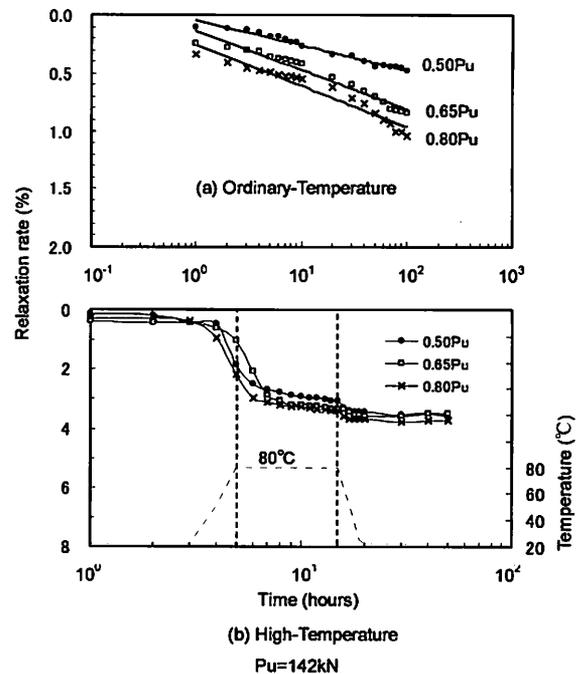
Fig.2 Relaxation curve of CFRP cable
