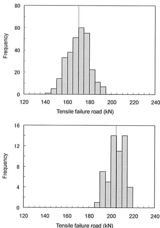
Fig.8 Frequency distribution of tensile failure load
