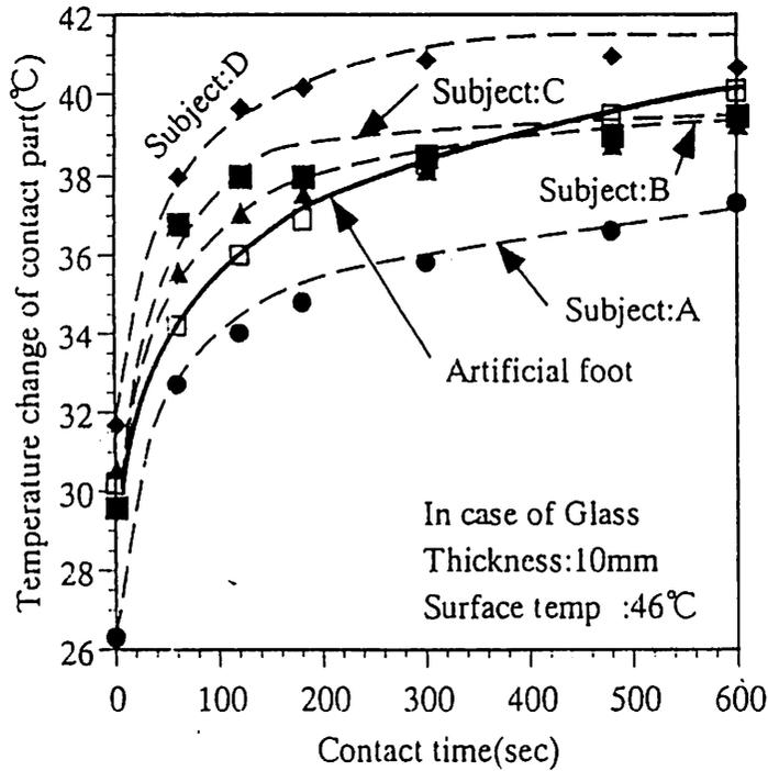
Fig.7 Temperature of contact part of artificial foot and palm of subject
