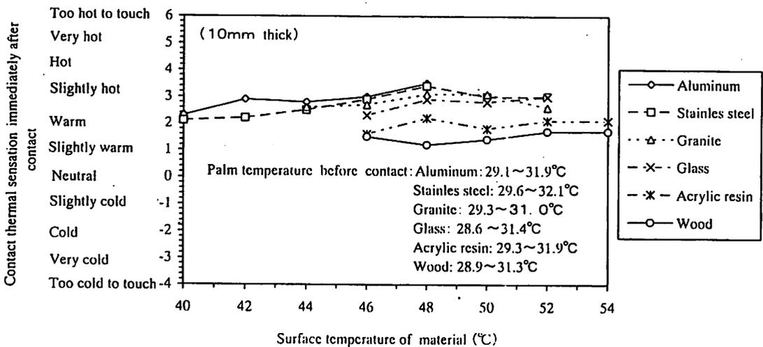
Fig-3 Relation between the surface temperature of material and the contact thermal sensation immediately after contact. (Average)
