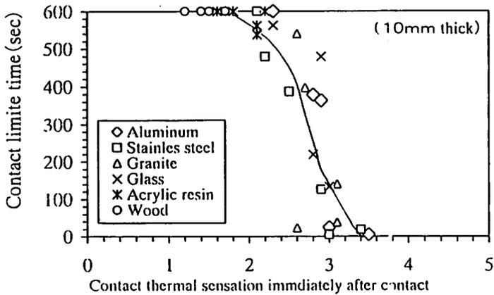
Fig-6 Relation between contact thermal sensation immediately after contact and the contact limit time
