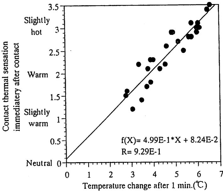
Fig.9 Relation between the temperature change after 1 min. and the contact thermal sensation immediatery after contact
