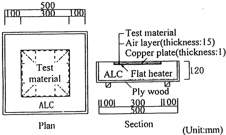
Fig.1 Heating unit for test material
