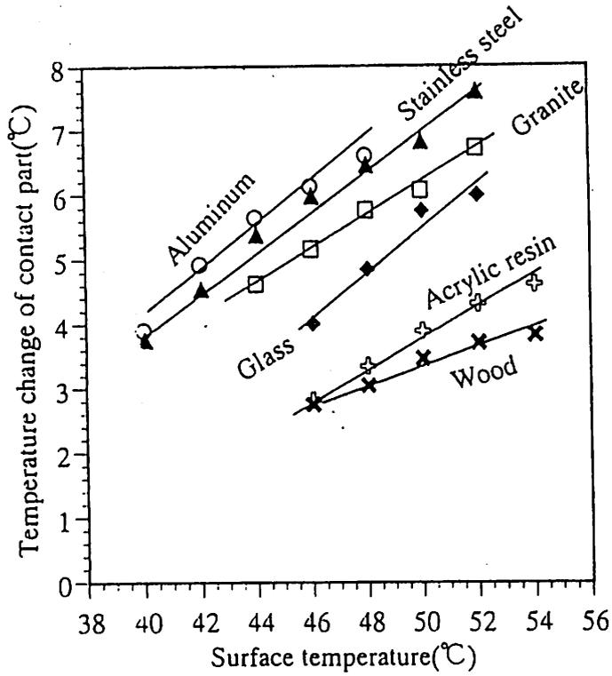
Fig.8 Relation between the surface temperature of material and the temperature change of contact part
