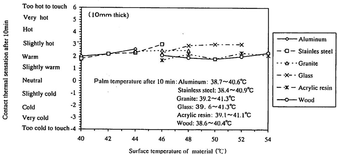
Fig-4 Relation between the contact thermal sensation after 10 min. and the surface temperature of material (Average)
