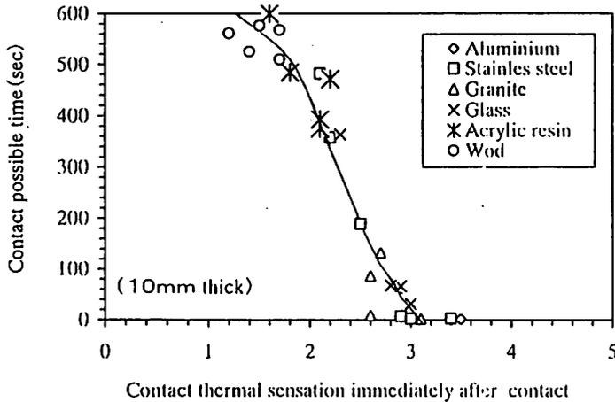
Fig-5 Relation between contact thermal sensation immediately after contact and the contact possible time
