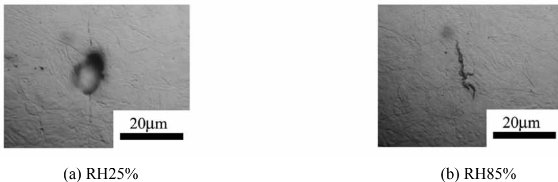
Figure 7. Feature of crack of Steel C (←→ Axial direction)
