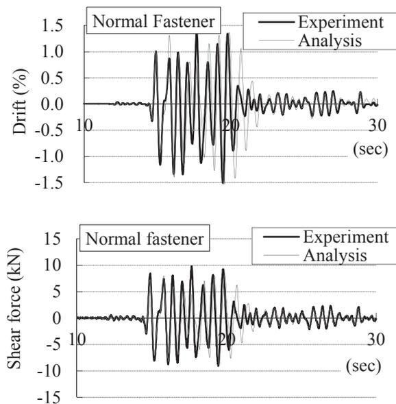
**Figure 10:** Time history of the case with normal brace fasteners under 30% of JMA Kobe wave
