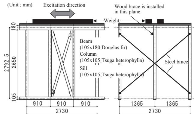
Figure 2: Wood frame for shake table test
