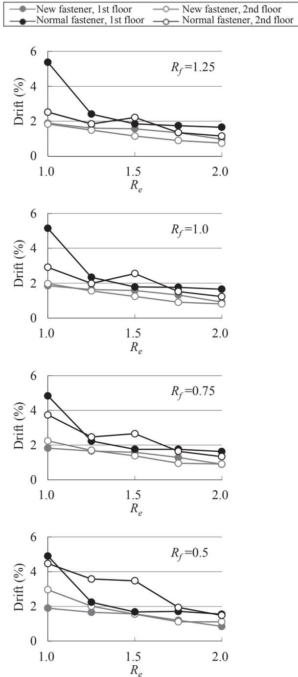
**Figure 12:** Maximum response drift of two-storied analysis model under JMA Kobe wave
