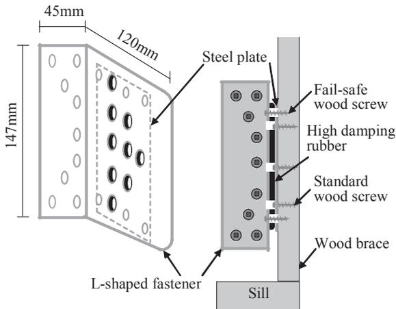
Figure 1: New developed brace fastener
