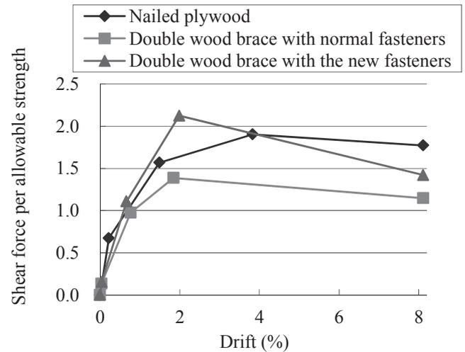
**Figure 15:** Shear force per allowable shear strength of shear walls
